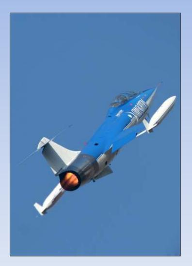
The Lockheed F-104 Starfighter is the highest performance, single-engine jet fighter ever made. The F-104 is powered by a single General Electric J79-GE-11A engine capable of generating in excess of 17,000 lbs of thrust and exceeding Mach 2. For perspective, that's roughly equivalent to 36,000 horsepower, or more than the entire starting line-up at the Daytona 500.
