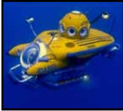
Idabel is designed to safely transport three people to a depth of 3000 feet (915 meters) below sea level. Her safety features include twin ballast compartments, twin high-pressure air systems, a 350 pound droppable lead weight and fully redundant propulsion systems. She has no rudder, dive planes or other moving parts to jam and is equipped to provide three days of emergency life support. Features include:
